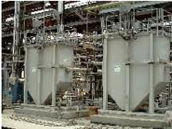
Composite separators with flotation and sedimentation function.
